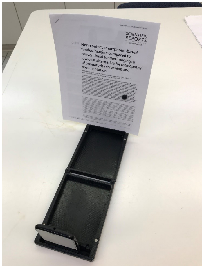
A full sheet of paper is held in place with fully extended stand back and magnet. Phone is positioned optimally from document.
