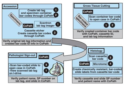
**IFigure 21** An "electronic kanban" of bar codes connects work cells and defines, standardizes, and mistake-proofs the work processes of surgical pathology. Bar code number key: (1) laboratory requisition (lab tag), (2) specimen container, (3) tissue cassette, and (4) glass slide. Manual quality control checks are described in the lower shaded box of each work station. SP, surgical pathology.
