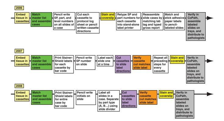
**Figure 11** Process flow map of the work steps in the histology laboratory of the 3 workflow conditions of simple bar-coded (2006), bar code work-specified processes (2007), and lean evolved bar code work-specified processes (2008). Processes within the same colored boxes are identical, and processes within uncolored boxes differ. SP, surgical pathology.
