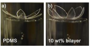
Figure 2: (a) PDMS without PAAm layer. (b) Bilayer samples with 10 wt% initial monomer concentration.
