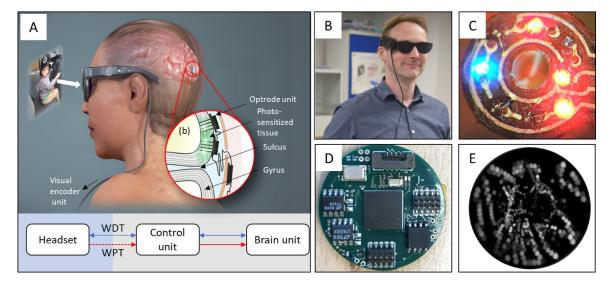
Fig. A. The concept of the visual cortical prosthesis. B. The headset unit. C. The brain unit. D. The control unit. E. The processed image.
