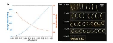
Figure 1: Characterizations of hydrogels and curvature measurement of bilayer strips. (a) Young's modulus and expansion strain of hydrated hydrogels with different AAm initial concentrations. (b) Hydrated bilayer strips (17 mm x 2.5 mm (length x width) with different AAm wt%.
