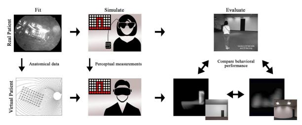
Fig. 1: Virtual and real patients for bionic vision. Top: Real patient performing a door locating task. Bottom: Simulated device created by matching anatomical and perceptual measurements from real patients being used to perform virtual and augmented reality versions of the same task
