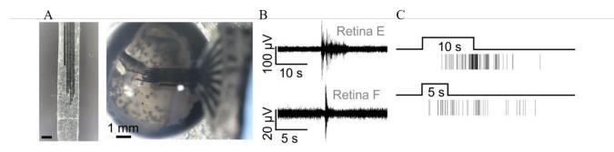
Figure 1. (A) SoftC probe (left), probe placed inside the eye (right). (B) Spontaneous retinal activity recorded in enucleated eye. (C) Evoked retinal spikes recorded in enucleated eye to 405 nm illumination.
