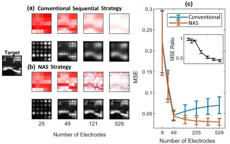
**Figure 1:** The effect of the maximum safe electrode amplitude (Method I). a) and b) The electrode amplitudes and retinal activity using fixed electrode spreads (visible in the left-most column). c) The mean squared error (MSE) across 32 images.
