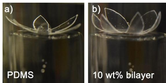
Figure 2: (a) PDMS without PAAm layer. (b) Bilayer samples with 10 wt% initial monomer concentration.
