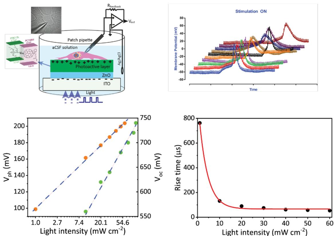
Figure: (a) Photoelectrode and a patch-clamp set-up schematic, (b) Membrane potential under light-pulse for single cell, (c) light-controlled variation of photovoltage and open-circuit voltage, and (d) light-controlled switching speed.
