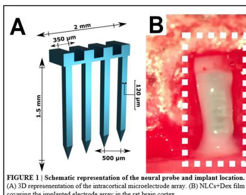
**FIGURE 1 | Schematic representation of the neural probe and implant location. (A) 3D representation of the intracortical microelectrode array. (B) NLCs+Dex film covering the implanted electrode array in the rat brain cortex.**
