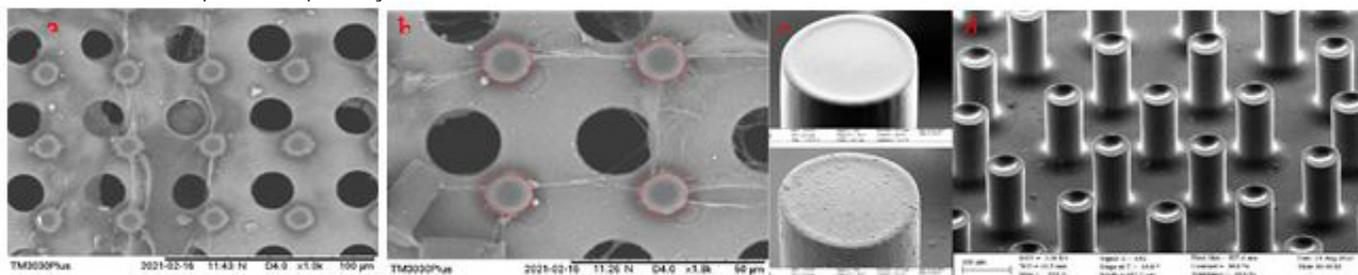
**Figure 1:** (a) PC12 cells on the surface of a photovoltaic Si chip with 3D carbon pillars. Cell nuclei are indicated by red circles (b) and seem to be placed at the very tip of the carbon pillars. 3D carbon pillars (c, top) with polydopamine (c, bottom) passivation and after removing the passivation layer at the tip of every carbon pillar using a laser (d).
