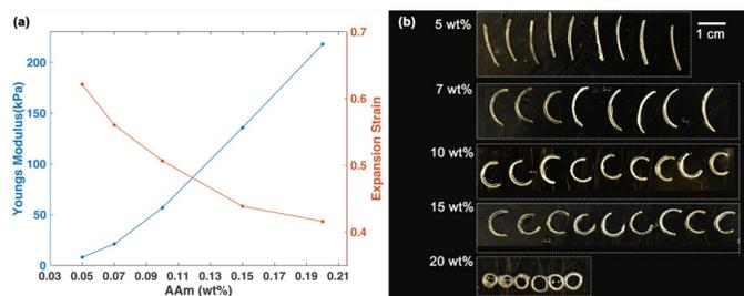
Figure 1: Characterizations of hydrogels and curvature measurement of bilayer strips. (a) Young's modulus and expansion strain of hydrated hydrogels with different AAm initial concentrations. (b) Hydrated bilayer strips (17 mm x 2.5 mm (length x width) with different AAm wt%.
