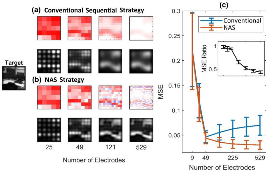
**Figure 1:** The effect of the maximum safe electrode amplitude (Method 1). a) and b) The electrode amplitudes and retinal activity using fixed electrode spreads (visible in the left-most column). c) The mean squared error (MSE) across 32 images.
