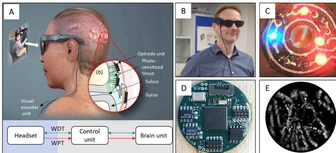
Fig. A. The concept of the visual cortical prosthesis. B. The headset unit. C. The brain unit. D. The control unit. E. The processed image.
