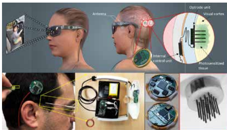
Fig. 1. (top) The 3D concept image of a full wireless multi-colour optogenetics visual cortex implant prosthesis. (bottom, left to right) The implantable control unit, the exemplar headset and external unit, and the optrode array from the CANDO project.
