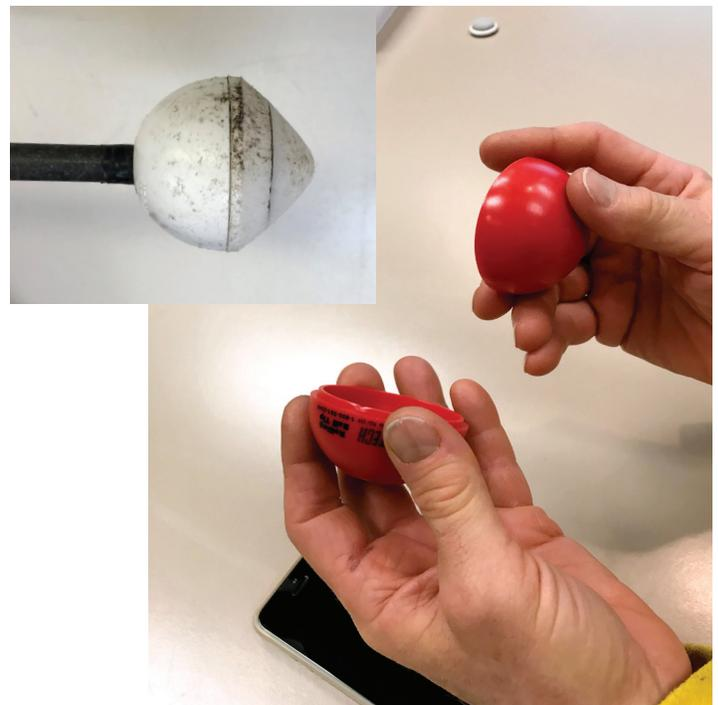
Nino Pacini demonstrates the traditional two-piece, injection molded ball tip. Terminal wear on a standard ball tip. The worn shape is more effective than a ball shape.
