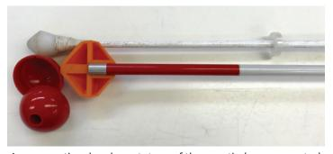
A cross-sectional early prototype of the new tip (orange, center) next to a disassembled ball tip and worn "mushroom tip".
